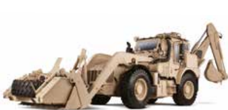
Built in Savannah, the fully armored JCB High Mobility Engineer Excavator (HMEE) is the world's toughest backhoe.
