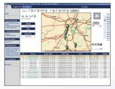
Machine tracking during transport - When your machine is transported, KOMTRAX<sup>TM</sup> sends travel messages to the web site or by e-mail to inform you of its progress, and confirms when it reaches its destination.
