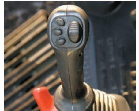
Joysticks with proportional control button for attachments
