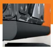
■ Reinforced D-channel side frames provide maximum cab and component impact protection.
