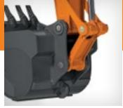
■ Tungsten-carbide-coated surfaces protect the critical bucket-to-arm joint.
