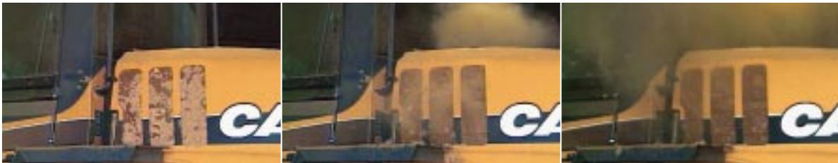
*In work environments with high levels of dust or airborne debris, the D Series optional reversible fan provides a time-saving solution to cleaning the cooling module.*
