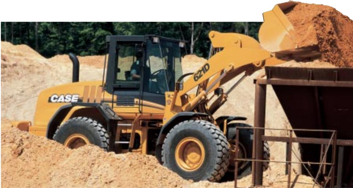
Newly designed D Series buckets more efficiently slice into the pile and fill more quickly and fully than ever before. The new bolt-on cutting edge has been redesigned to penetrate the pile like a knife.
